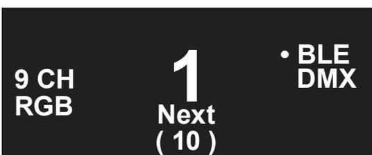
☞ A little white dot in front of „BLE“ in the ROXX® fixtures display indicates a working connection and incoming control signal from the app.
