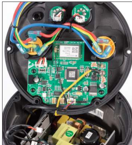
Connection terminal, control board and power supply in the rear section
