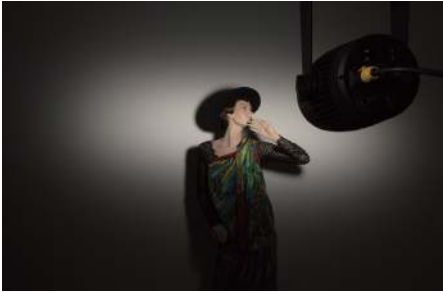
Light image of the wide, asymmetrical lens (EW) To ensure that the light field does not end outside the image, the distance from the spotlight to the wall was only 1.8 m in this case
