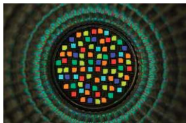
LEDs in TW+ 10 red, 10 green, 10 blue, 20 amber, 10 cyan and 20 lime and the corresponding spectrum
