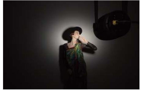
Light image of the narrow asymmetric lens (EN) - The distance to the wall has remained the same for comparison purposes
