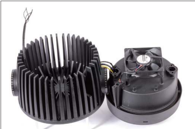
Left and right of the fan Sealing glands for the connecting tubes to the front LED module. Where the gap or a missing cooling fin can be seen, the plastic fin mold with the W-DMX antenna inside is placed
