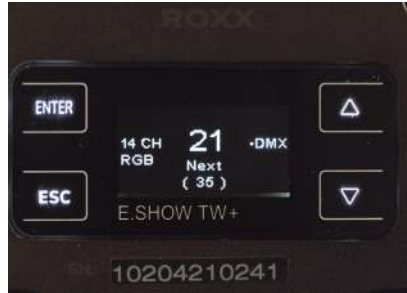
Menu operation Illuminated touch keys and clear graphic display
