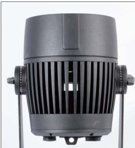
Three-part Front chamber on top with the reflector, LED and LED driver board, the open middle part formed mainly by the cooling fins, for cooling with fan. The last third is the rear chamber with connection terminal, control board and power supply unit
