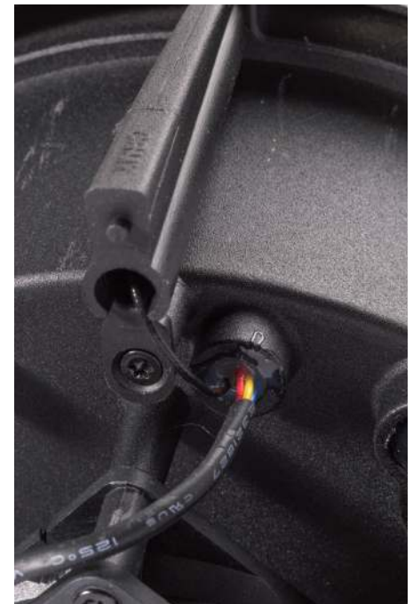
Antenna for W-DMX hidden in a plastic cover, in the design of a cooling fin
