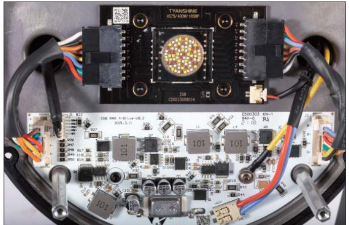
LED engine of the E.Show FC with the driver board
