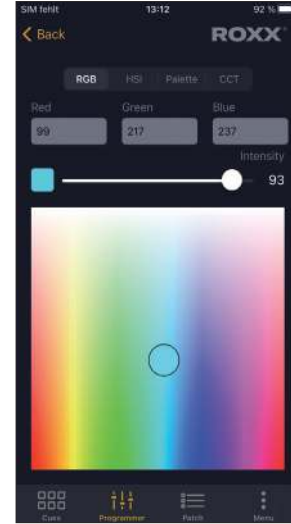
App for iPhone/ iPad replaces the remote control via Bluetooth a device is connected that controls other devices via DMX or W-DMX
