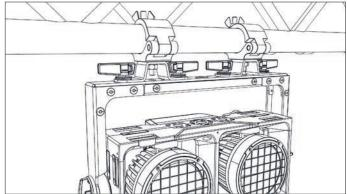
**d. With 2x Omega Bracket** Max. Tension Load: 90kg Max. Torsion Load: 5.943 Nmm
