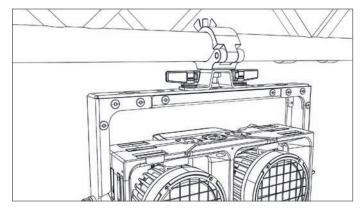
**c. With 1x Omega Bracket** Max. Tension Load: 51kg Max. Torsion Load: 4.768 Nmm
