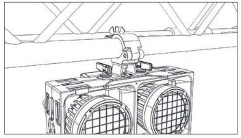
Max. Tension Load: 90kg Max. Torsion Load: 18.703 Nmm
