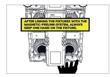
2. Pre-Link Magnets on top and side help to allign the fixtures due cluster process and giving support operation for convenient and save interlocking.
