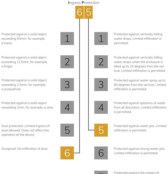
Protected against the impact of being immersed in water between 15cm and 1m for 30 minutes.
