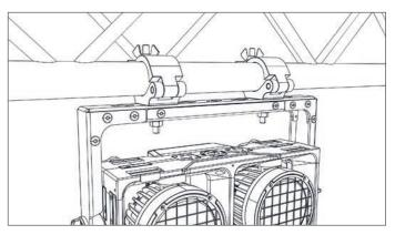
**b. With 2x Mounting Clamp** Max. Tension Load: 77kg Max. Torsion Load: 7.308 Nmm
