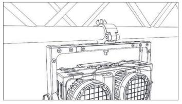
**a. With 1x Mounting Clamp** Max. Tension Load: 40kg Max. Torsion Load: 4.414 Nmm
