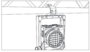
**e. YOKE 2.2 with 1x Mounting Clamp** Max. Tension Load: 88kg Max. Torsion Load: 8.238Nmm
