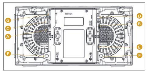
**A: Mains In:** IP65 Power input connector with rubber sealing cap.Connect using the provided power cable (when not in use, always close with rubber sealing cap).
