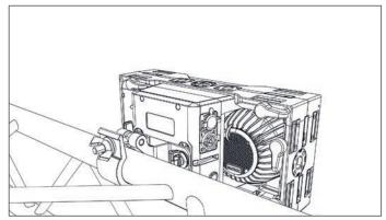
Max. Tension Load: 90kg Max. Torsion Load: 14.201 Nmm
