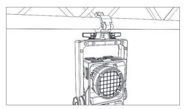
**f. YOKE 2.2 with 1x Omega Bracket** Max. Tension Load: 66kg Max. Torsion Load: 6.476Nmm
