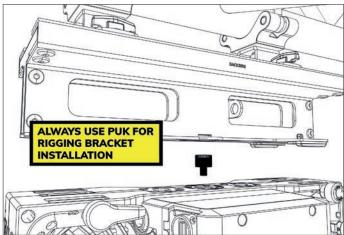
For seemless connection of multiple Blinders, to avoid gaps due to bracing of the truss structure by variable, sliding mounting positions.
