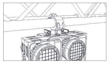
Max. Tension Load: 90kg Max. Torsion Load: 14.500 Nmm
