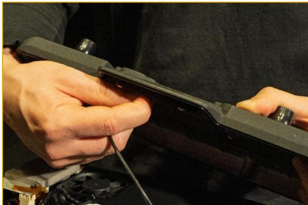
9. **Close the bottom plate** of the fixture. Ensure the grounding cable is not pinched or damaged.
